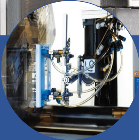
2-component production with turntable technology
